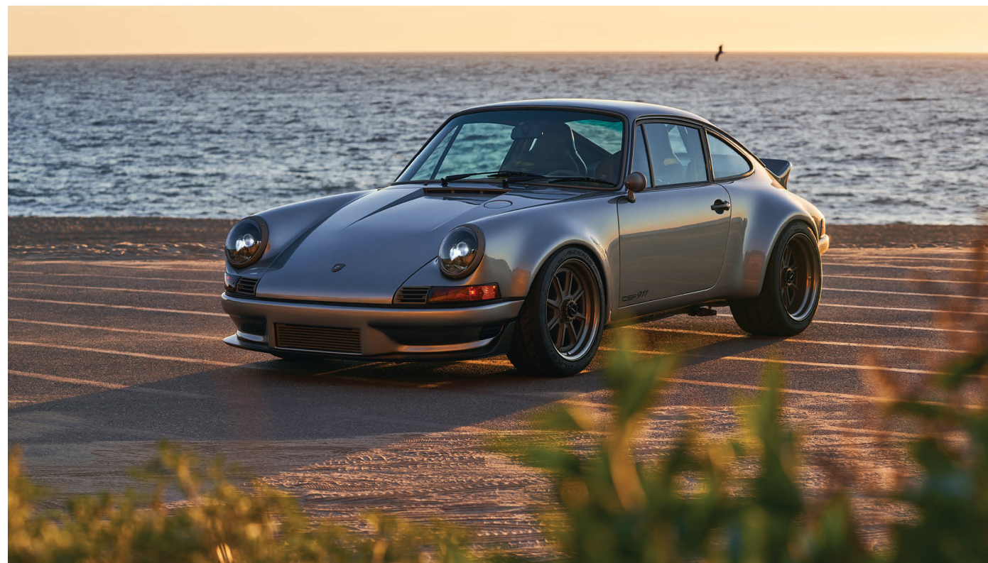
Fender flares accommodate the 911 SC's Falken Azenis RT 660 275/40ZR17 rear tires. A custom fuel bib prevents fuel spillage in the bespoke gas cap on the hood.
