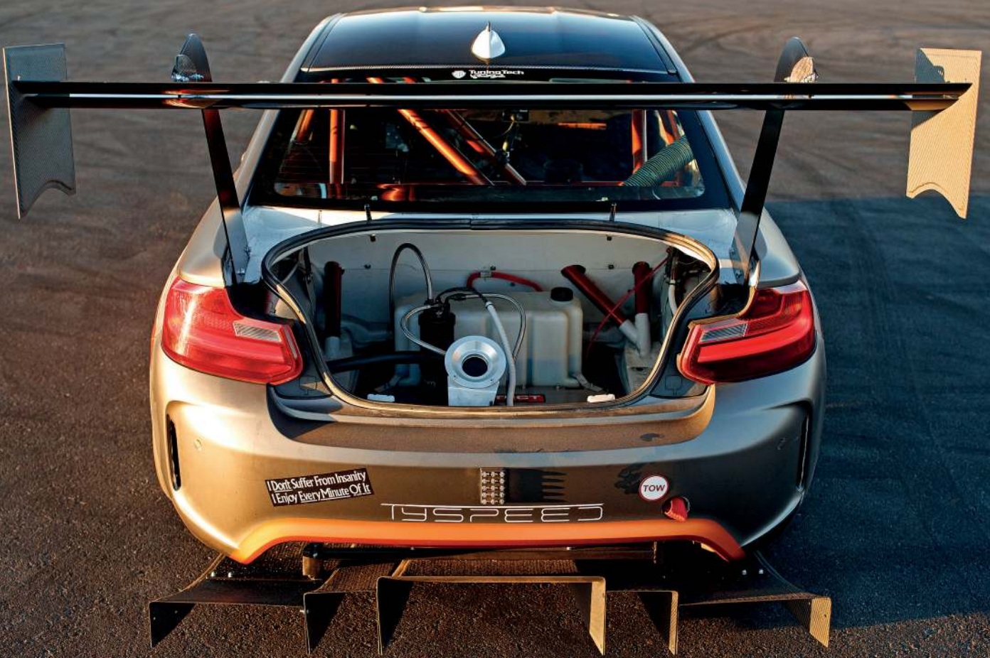
Boot houses fuel setup with dry break filling system
